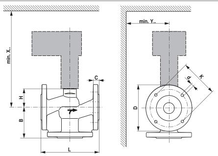
X/Y: Minimum distance with respect to the valve centre.
